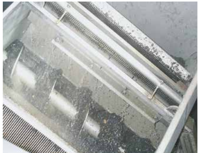
Floating and suspended material is retained in the screen basket. The tines mesh into the basket bars and ensure a complete automatic cleaning.
