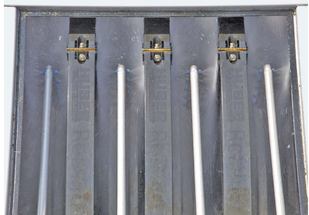
Backwashing of filter discs with filtrate – no external wash water required.
