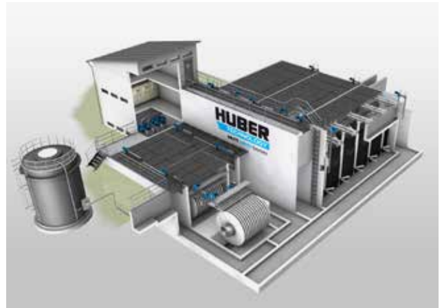
HUBER Pile Cloth Media Filter RotaFilt®, Ozonation and HUBER Active Carbon Filter CONTIFLOW® GAK.
