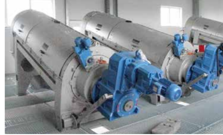
HUBER Screw Press units for sludge treatment – best dewatering performance and highest volume reduction for lower disposal costs.
