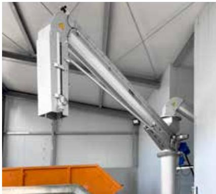
Rotating distribution screw Ro8 TC for dewatered sludge.
