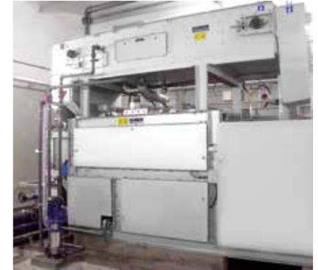
The HUBER Bogenpress B-PRESS can be combined with the HUBER Belt Thickener DrainBelt unit to further increase capacity.
