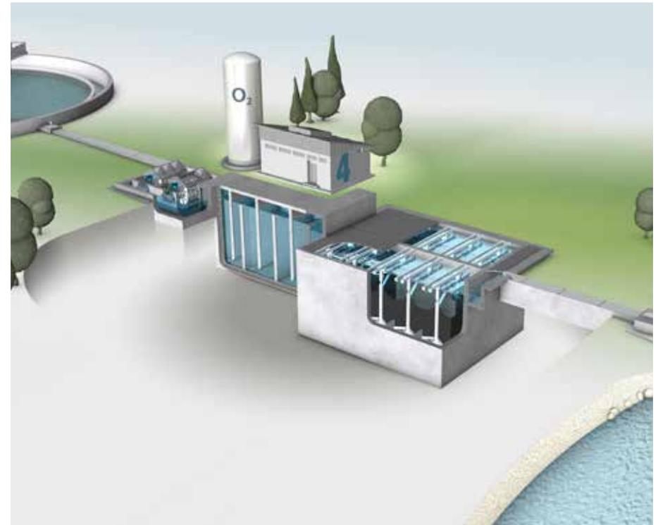
Advanced wastewater treatment for the removal of trace substances with the combined process of ozonation and downstream HUBER Activated Carbon Filter CONTIFLOW® GAK.
