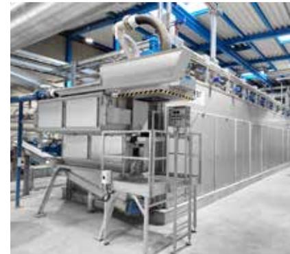
*HUBER Belt Dryer BT for sewage sludge drying up to > 90% DR.*
