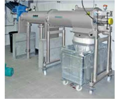
HUBER Sludg cleaner STRAINPRESS® – continuous pressurised coarse material separation.
