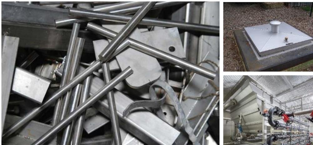
Fig. 19: HUBER manufactures products and machines for water and wastewater every year from approx. 4,500 t stainless steel. Reducing waste is a prerequisite for cost-optimised and resource-saving production when processing high-quality materials. HUBER therefore nests the parts to be manufactured from stainless steel with state-of-the-art CAM software for all orders. 100% of the stainless steel waste generated during production is recycled.
