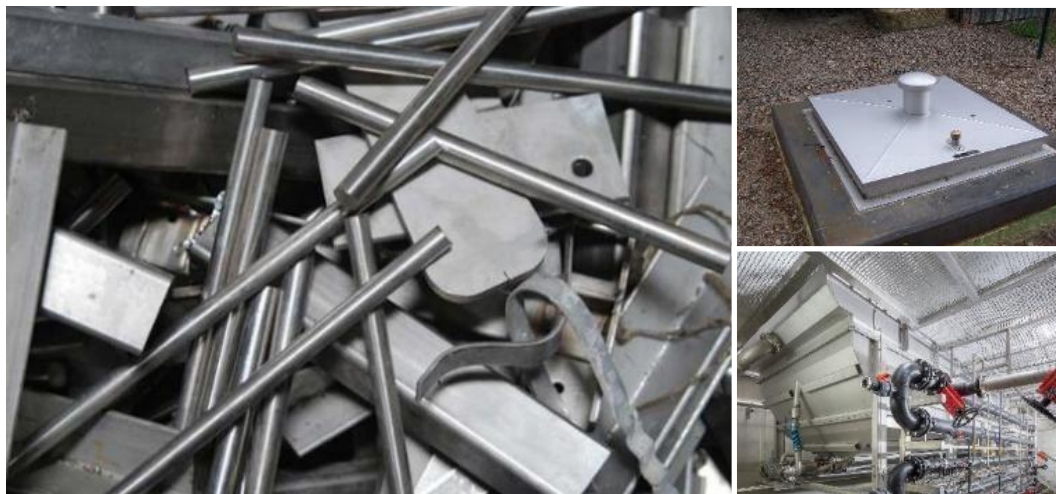
Fig. 24: A large proportion of our waste consists of stainless steel. Reducing waste is a prerequisite for cost-optimised and resource-saving production when processing high-quality materials. HUBER therefore nests the parts to be manufactured from stainless steel with state-of-the-art CAM software for all orders. 100% of the stainless steel waste generated during production is recycled.
