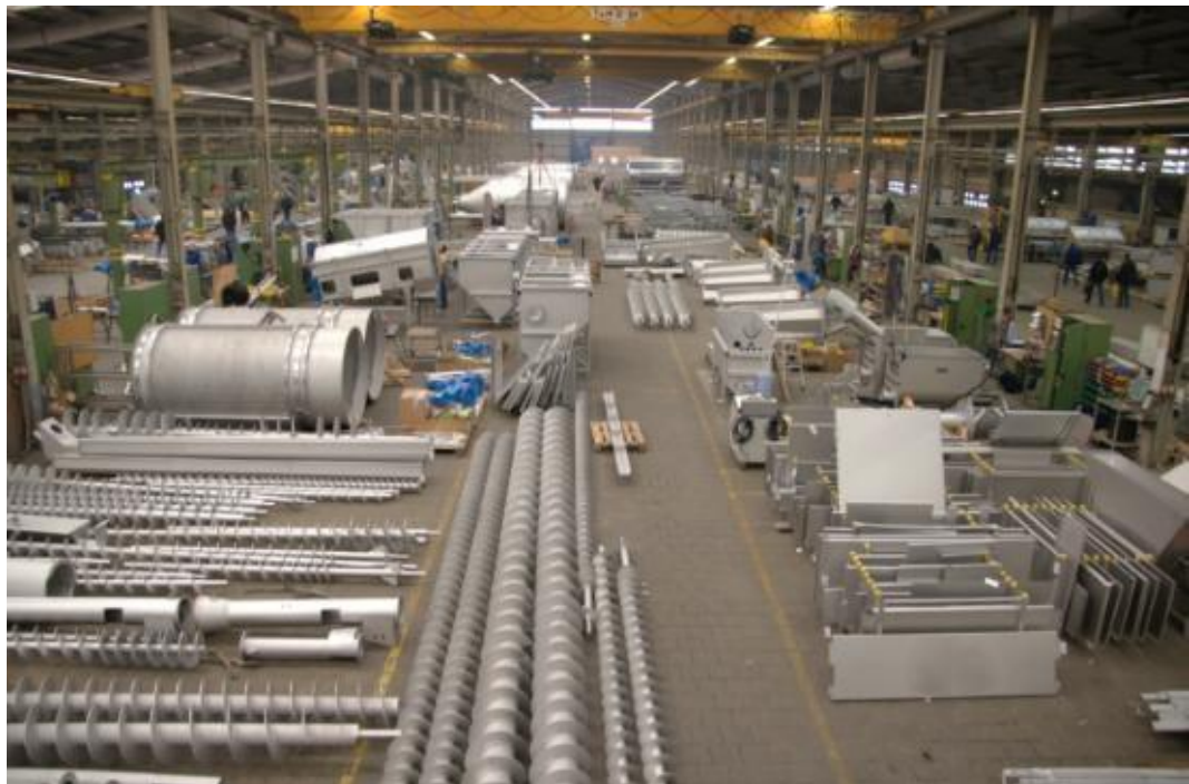
Fig. 29: HUBER SE processes approximately 4,500 t of stainless steel annually and from this manufactures different products for the field of water supply and wastewater disposal.
