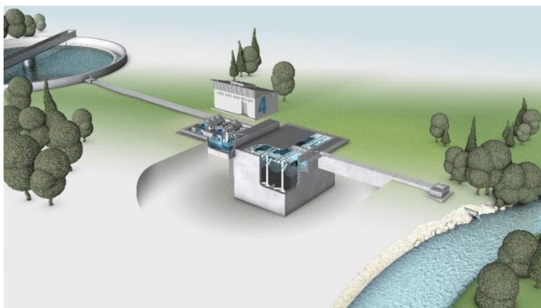
Fig. 21: HUBER has also developed solutions to treat water even further than usual. A so-called 4th treatment stage removes trace substances, such as pharmaceuticals, from the wastewater by adsorbing these substances to activated carbon.
