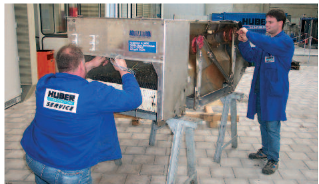
The factory repair team: repair and maintenance of a machine from another step screen manufacturer
