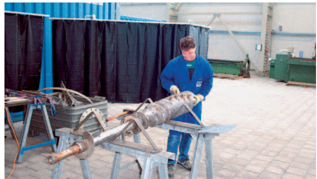
Overhaul of a used screw shaft
