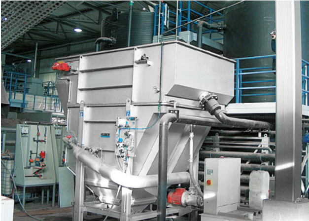
HUBER Dissolved Air Flotation HDF at a food waste treatment plant in Spain.
