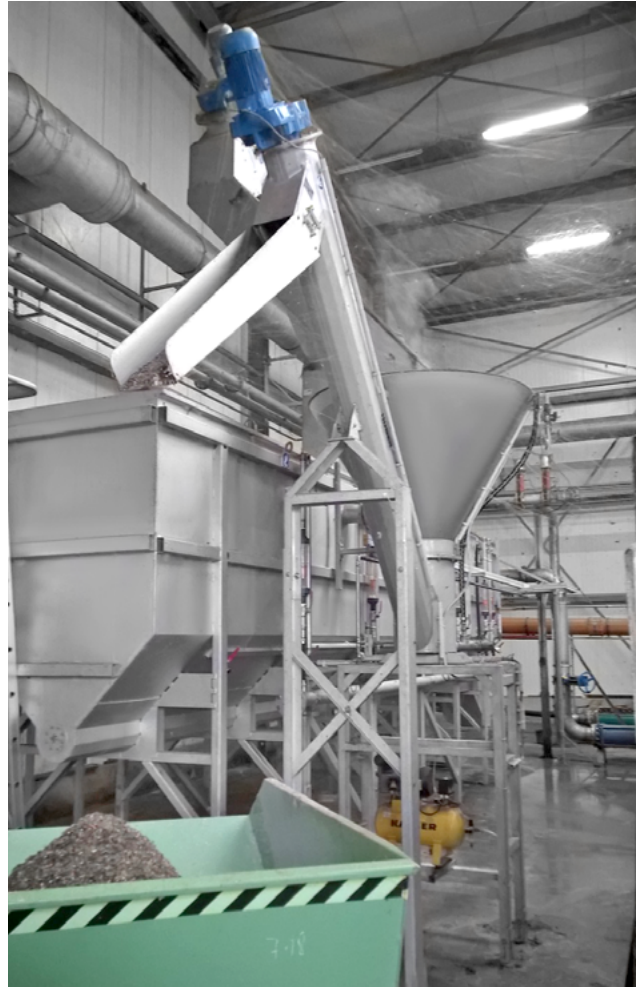
HUBER Grit Washing Plant RoSF G4E Bio at a German biowaste treatment plant.
