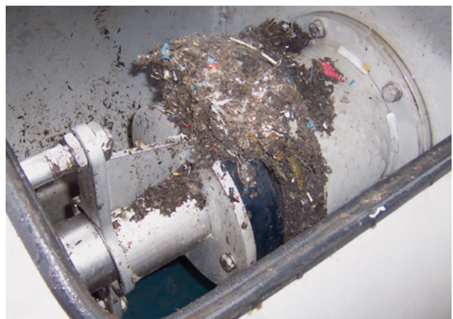
Separated and dewatered foreign matter from the HUBER STRAINPRESS® at a biological waste treatment plant in Germany.
