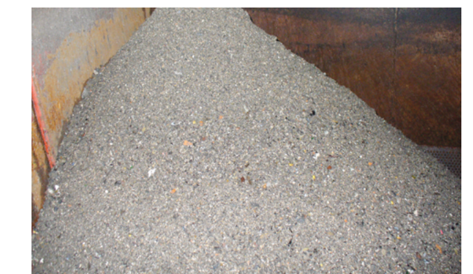
The product discharged from the HUBER Grit Washing Plant RoSF G4E Bio: washed mineral material.
