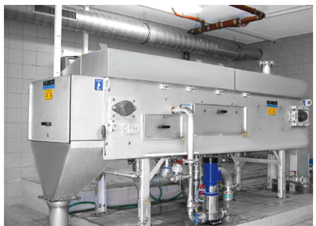
Belt washing with filtrate water as spray water.
