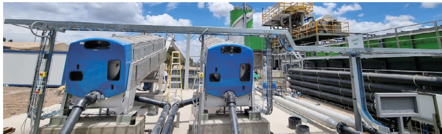
HUBER Screw Press units for sludge treatment – best dewatering performance and highest volume reduction for lower disposal costs.
