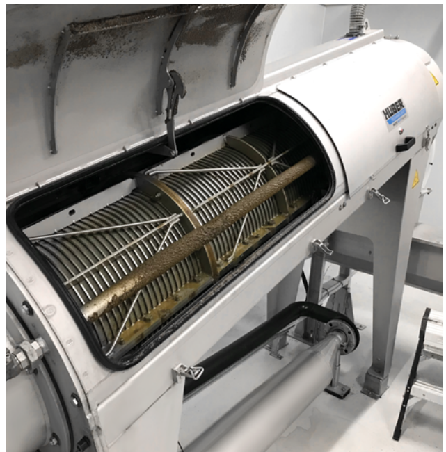
HUBER Screw Press for dewatering of residual sludge from onshore fish farms (salmon production) – reduced disposal costs.
