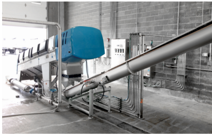
HUBER Screw Press units for sludge treatment – best dewatering performance and highest volume reduction for lower disposal costs.
