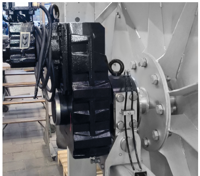
Low-maintenance chain drive on the HUBER Drum Screen LIQUID.
