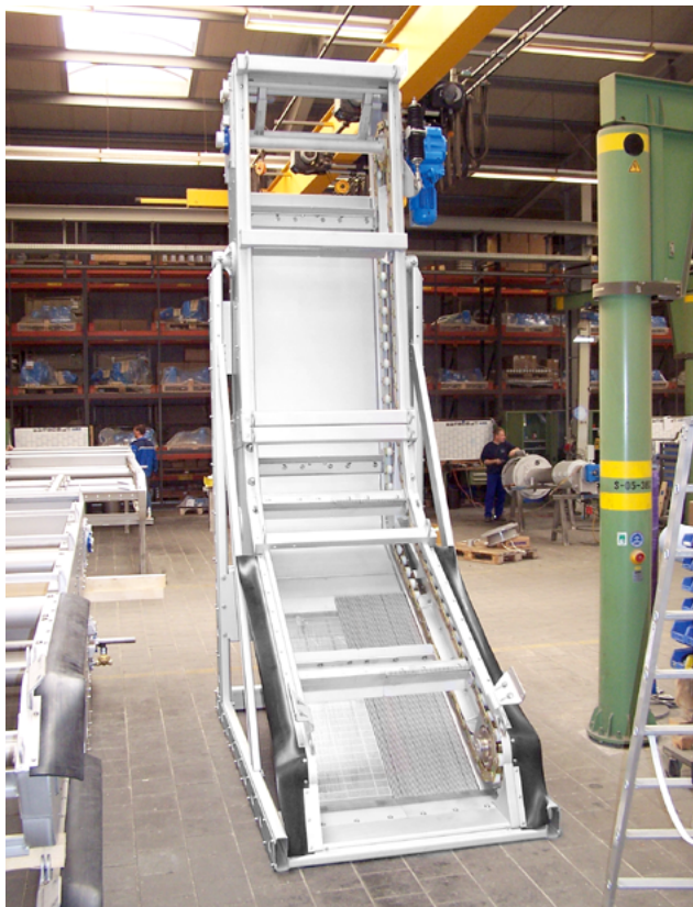
HUBER Rake-Max® HF unit in our factory before delivery: The flat bottom section which provides favourable hydraulic conditions is clearly visible.
