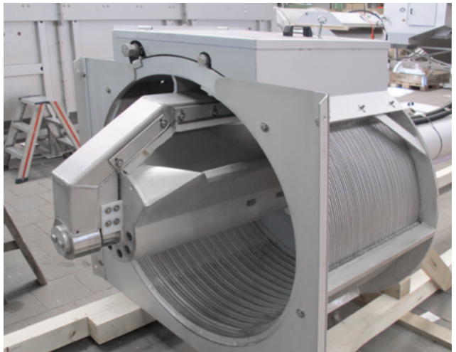
HUBER Fine Screen ROTAMAT® Ro1 with screen basket cover to prevent that splash water escapes.
