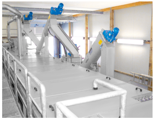
Odour-encased screenings discharge from the HUBER Complete Plant ROTAMAT® Ro5.
