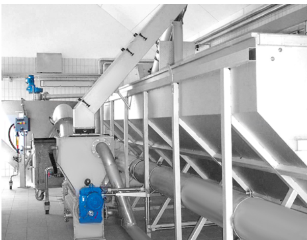
Intensive washing of screenings in a WAP® SL subsequent to a HUBER Complete Plant ROTAMAT® Ro5.
