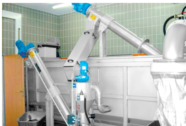
Classifying screw with subsequent HUBER Coanda Grit Washer RoSF4 T.
