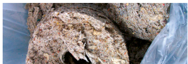
Washed and compacted screenings – the ideal fuel.
