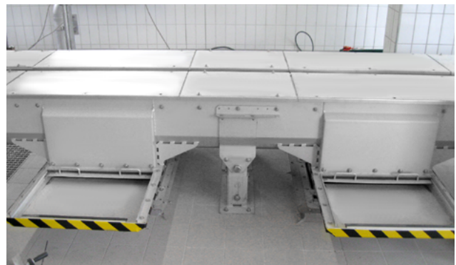
Manually operated slide gate.
