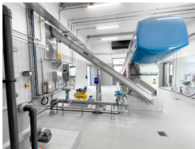
Inclined conveyor supply downstream of a HUBER Screw Press Q-PRESS®.
