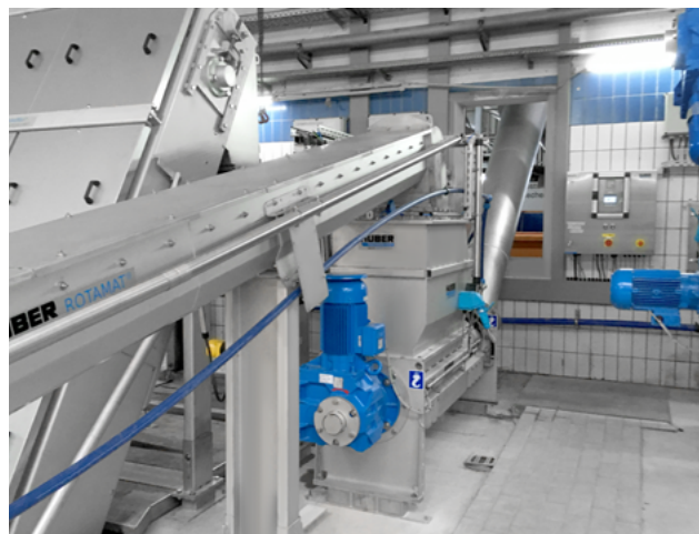
Conveyor solution for mechanical pre-treatment of unpressed screenings.
