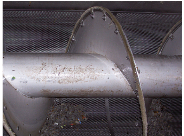
Gentle automatic cleaning of the semi-circular perforated plate.
