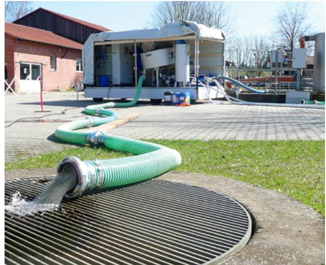
Mobile HUBER Disc Thickener S-DISC mounted on a car trailer, clear filtrate water runs off in the foreground.
