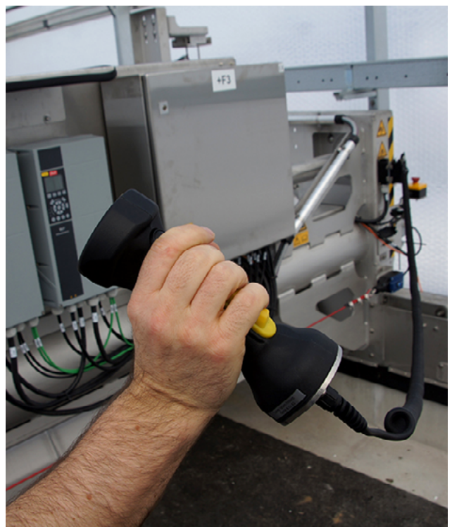
Enabling button for safe maintenance.
