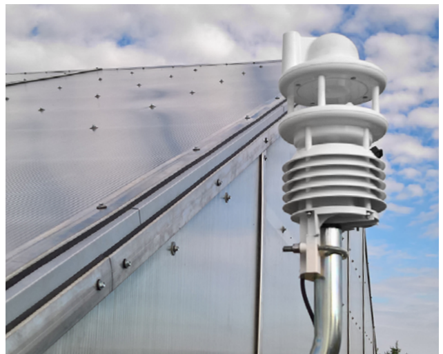
The weather station delivers measurements for an automatically regulated climate control system.
