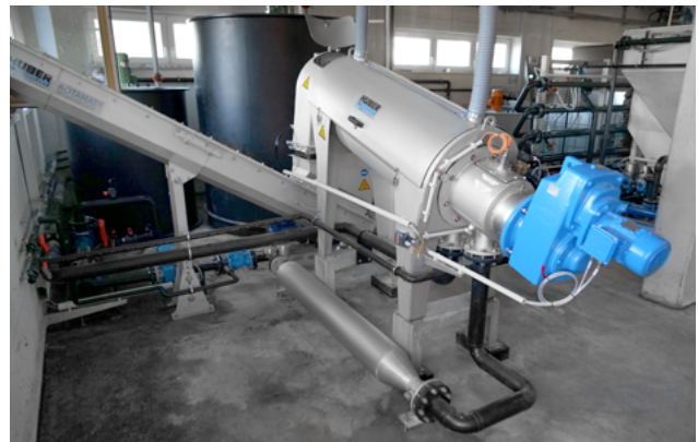
HUBER Screw Press Q-PRESS® for process sludge dewatering in tanneries.
