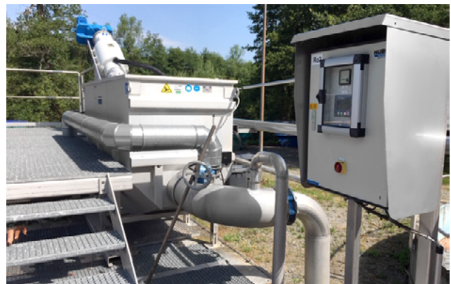
Process wastewater screening for textile fibre separation.
