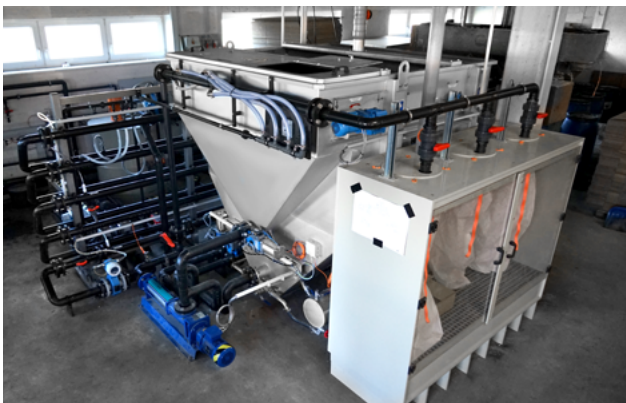
HUBER Pressure Relief Flotation HDF for process wastewater treatment in leather factories.
