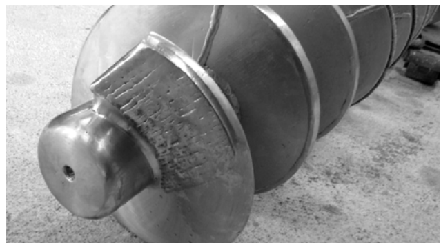
Advanced wear on a screw shaft.
